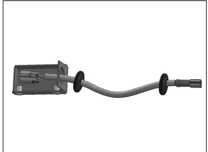
(Fig 9) Insert Harness Extension into driver/left Back Cover and plug into sensor in Housing
