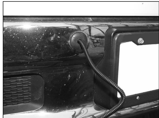
(Fig 11) Plug Harness into sensor harness
