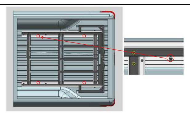
Step 4: Install the base of slide tray ① on the truck bed with hardwares ②③④⑤⑥
