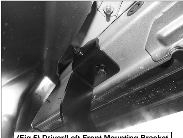
(Fig 5) Driver/Left Front Mounting Bracket attached to the front mounting location
