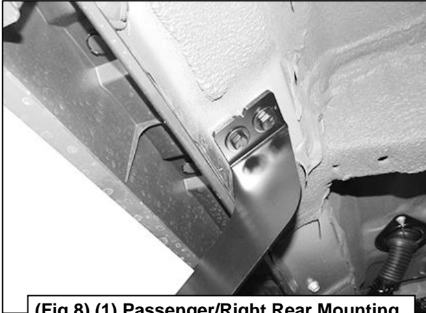
(Fig 8) (1) Passenger/Right Rear Mounting Bracket attached to the 3rd location
