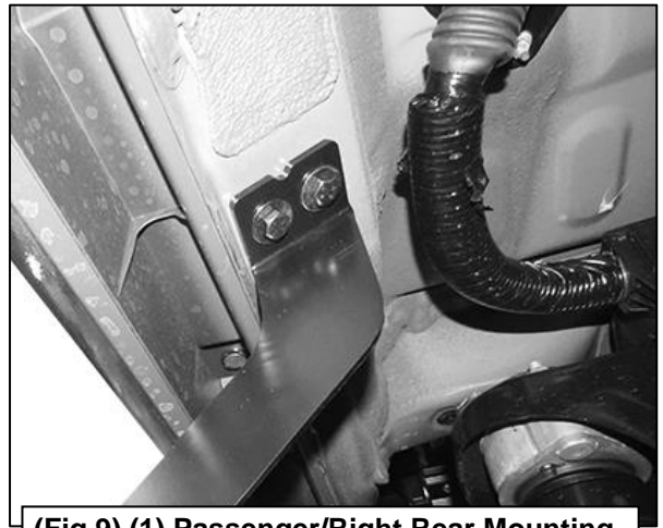
(Fig 9) (1) Passenger/Right Rear Mounting Bracket attached to the rear location
