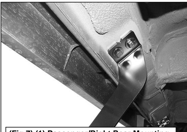
(Fig 7) (1) Passenger/Right Rear Mounting Bracket attached to the 2nd location
