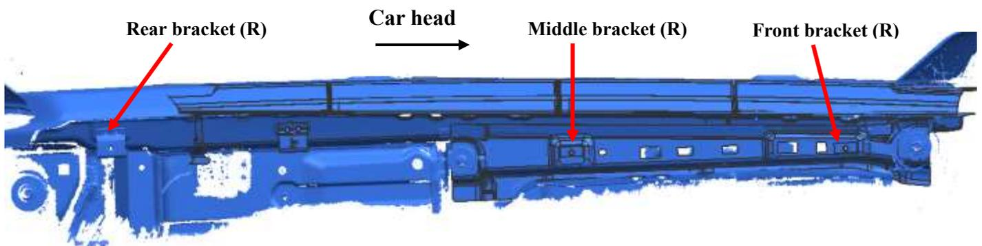
STEP2: Find the corresponding installation position of brackets in the figure (the picture shows the right side of the car).
