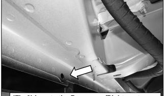
(Fig 9) Locate the Passenger/Right center mounting location. Line up the top of the Passenger/Right Center Mounting Bracket to the hole in the pinch trim. Mark the top slot for drilling. Use a 1/2" drill bit, not included
