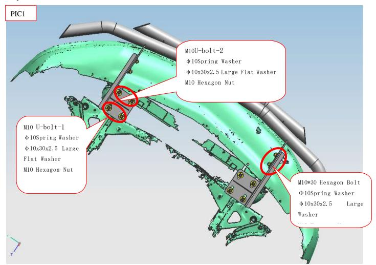
Step 3: Install the bar on the brackets, and tighten up all hardware after adjusting the brackets.
