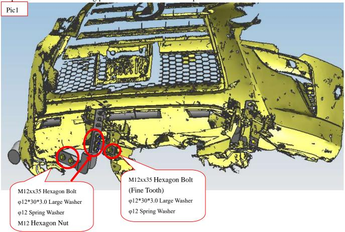
Step 3: Install the bar body on the bracket and adjust the mounting position of the bracket according to the position of the bar body.
