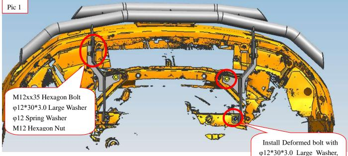
Install Deformed bolt with φ12\*30\*3.0 Large Washer, φ12 Spring Washer and M12 Hexagon Nut
