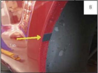
Fit a Tab (MT1-0014) circled over each of the four holes mentioned in Step 7, and enfolded around the metal lip.
