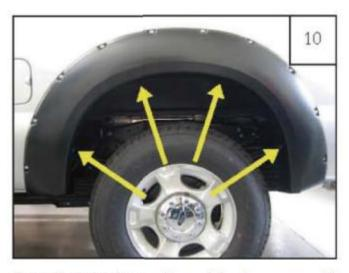
Keep flare on the position of fender, use a #2 Phillips screwdriver to install Screws (SWE1-0050) acrossing holes in flare and into clips, starting with the two top holes.
