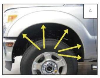
Using a 7/32' socket wrench to undo five factory screws and keep these screws for installing again.
