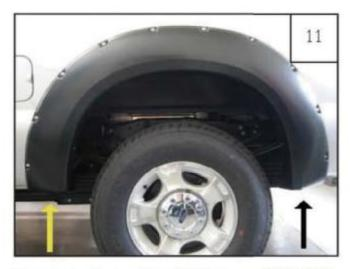
Fit up bolt, Washer(WA1-0010), Spacer(SP1-0008), Washer(WA1-0017) and Nut(NU1-0015) acrossing bottom two holes in flare and into factory holes with a 5/32' Allen Wrench and 3/8' socket.
