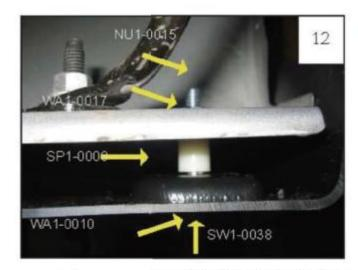
Actuate Screw from the bottom through the Washer and into flare, and fit up Spacer between flare and sheet metal, and then slide a Washer and then a Nut over the end of the Screw.
