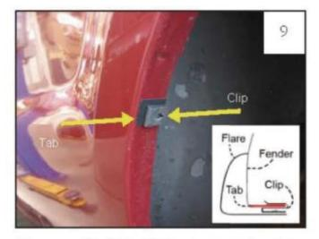
Fit up a Clip (CL1-0005) above each of the Tab (MT1-0014) done in Step 8.
