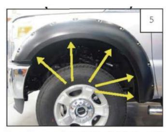
Keep flare on the position of fender, array factory holes and holes in the flare, and then using a 7/32' socket wrench to fit up factory screws through holes in flare and fender, starting with the top, centermost screw.
