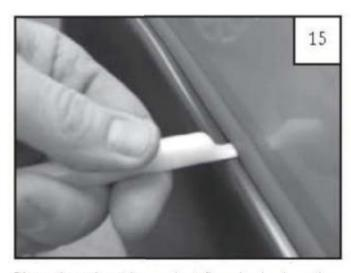
Place the edge trim against flare by by inserting straight end between edge trim and flare at one end and then slide around entire edge to the other end with the provided Edge Trim Tool (ET1-0002).
