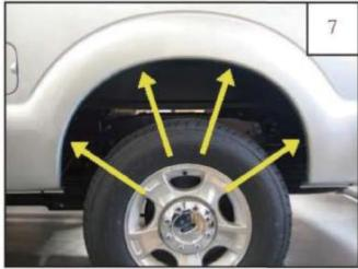
Keep flare to vehicle and ascertain the four holes in flares is lined up with four factory holes in the fender.
