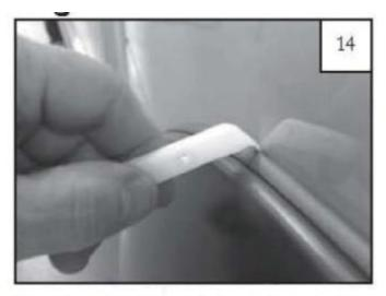
Place the edge trim against vehicle by hooking curved end beneath edge trim at one end of flare and then slide the outer edge of flare to the other end with the provided Edge Trim Tool (ET1-0002).
