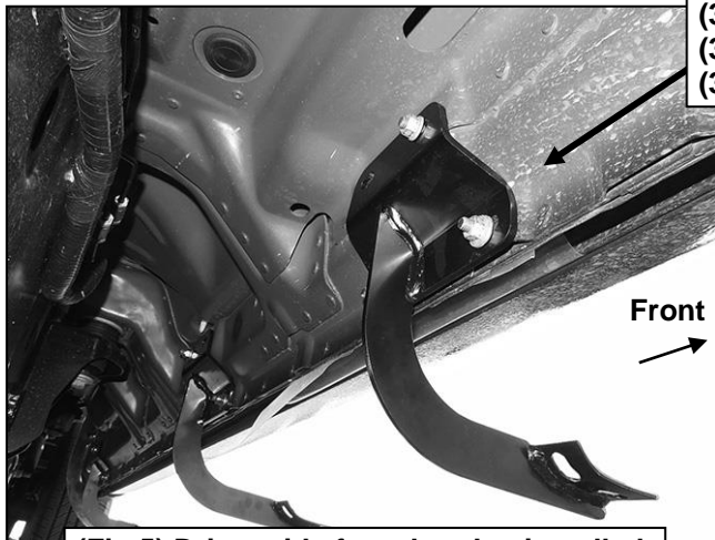
(Fig 5) Driver side front bracket installed
