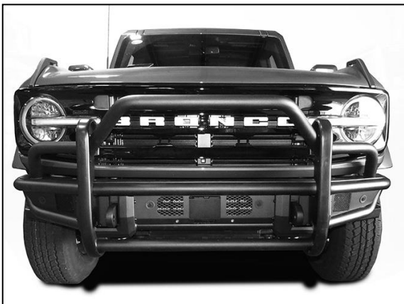
(Fig 9) Attach LED L Light Brackets above or below mount on Push Bar with hardware included in LD Bumper kit
