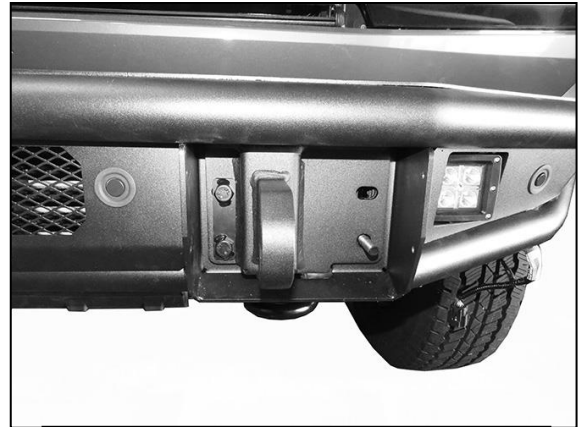
(Fig 4) Offset Shack Mount installed
