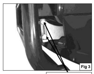
10mm x 35mm Hex Bolts 10mm Lock Washers 10mm Flat Washers 10mm Hex Nuts
