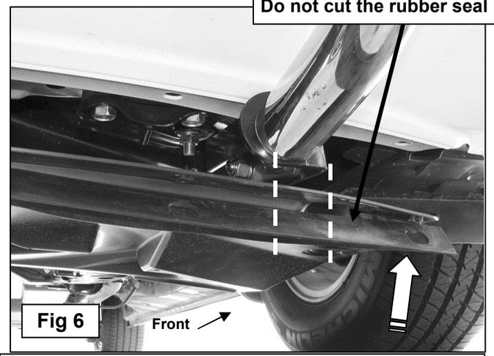
Hold the splash guard in position and mark the area to cut. Cut only the plastic splash guard. Do not cut the rubber seal.
