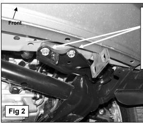
Due to tight tolerances, the holes in the factory frame support bracket may need to be filed slightly to provide additional clearance for the hex bolts after the Mounting Bracket is moved into position. DO NOT DAMAGE THE FINE THREADS ON THE FACTORY HEX BOLTS OR IN THE CROSSMEMBER
