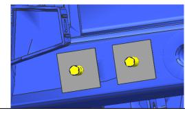
(Fig 2) Fix U Bolt M10x119.4 with (2) PVC Plastic blocks φ10
