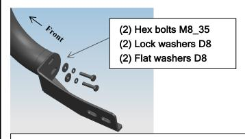
(Fig 5) Attach Driver/left guard tube bracket to bull bar
