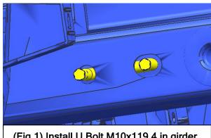
(Fig 1) Install U Bolt M10x119.4 in girder.
