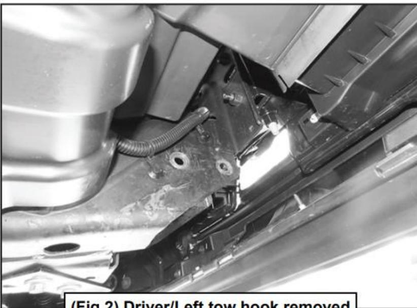
**(Fig 2) Driver/Left tow hook removed**
