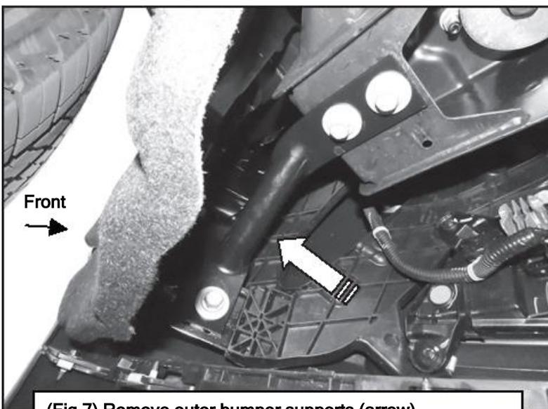
(Fig 7) Remove outer bumper supports (arrow)
