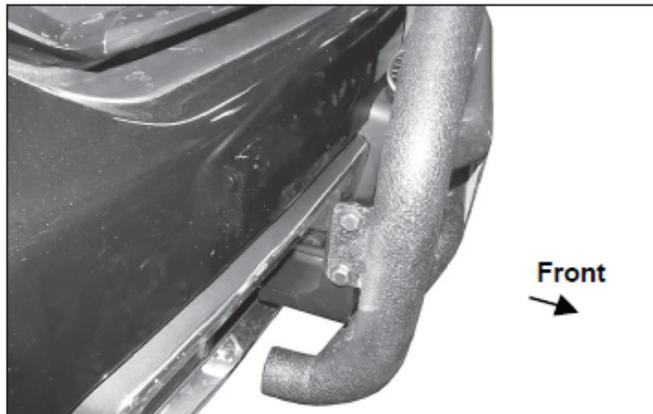
(Fig 19) Passenger/Right side complete installation
