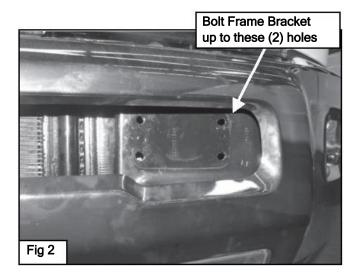
MAX T BULL BAR FOR 2010-2018 DODGE RAM 2500/3500 Use the factory tow hook hardware or the included: (2) 10mm x 35mm Hex Bolts (4) 10mm Flat Washers (2) 10mm Spring Washers (2) 10mm Hex Nuts Fig 4 Front Front Viewed from behind the (2) 10mm x 35mm Hex Bolts driver/left side of the bumper Fig 3 (4) 10mm Flat Washers (2) 10mm Spring Washers (2) 10mm Hex Nuts
