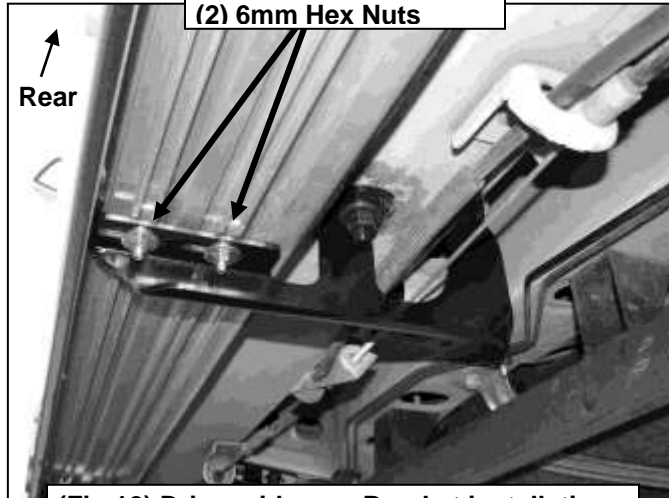
(Fig 12) Driver side rear Bracket installation
