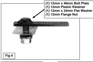
After inserting, rotate Bolt Plate 90-degrees to go across the slot or until Bolt Plate stops
