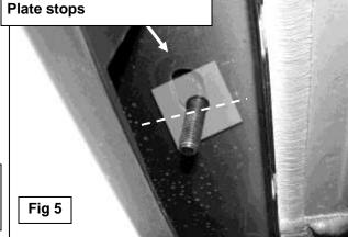
6mm x 25mm Hex Bolts 6mm x 18mm STD Flat 6mm x 22mm Large Flat Washers 6mm Nylon Lock Nuts
