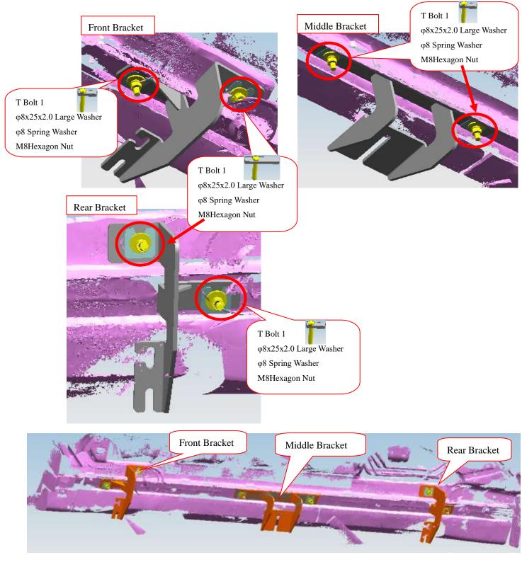
Step 3: Install the running boards on the brackets and then adjust them to the proper positions. Step 4: Check if all hard ware are installed and then fasten all to complete the installation.
