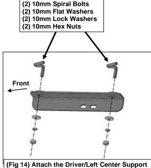
(Fig 14) Attach the Driver/Left Center Support Bracket to the (2) 10mm Spiral Bolts
