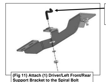
10mm Spiral Bolt 10mm Flat Washer 10mm Lock Washer 10mm Hex Nut
