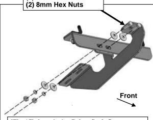
(Fig 15) Attach the Driver/Left Center Mounting Bracket to the Support Bracket
