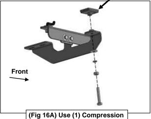
Plate to level the Bracket (Note use the Hex Nuts as adjusters)
