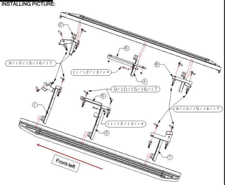
Step 1: Preview the approximate position of the body scan data and bracket in the picture below, and then install the brackets according to the actual car picture.
