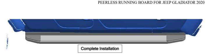
STEP4: After the running boards are adjusted to the appropriate position, lock all the standard parts. The installation position and manner of the left side brackets are the same as that of the right side.
