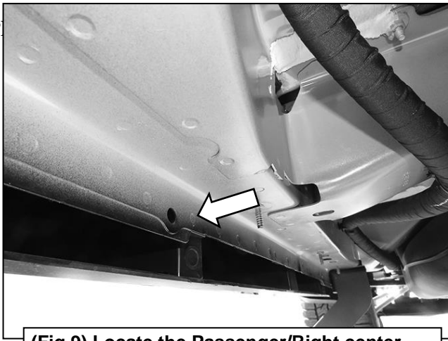
(Fig 9) Locate the Passenger/Right center mounting location. Line up the top of the Passenger/Right Center Mounting Bracket to the hole in the pinch trim. Mark the top slot for drilling. Use a 1/2" drill bit, not included
