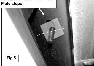
6mm x 25mm Hex Bolts 6mm x 18mm STD Flat 6mm x 22mm Large Flat Washers 6mm Nylon Lock Nuts
