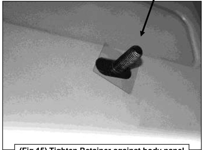
(Fig 15) Tighten Retainer against body panel
