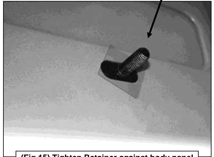
(Fig 15) Tighten Retainer against body panel
