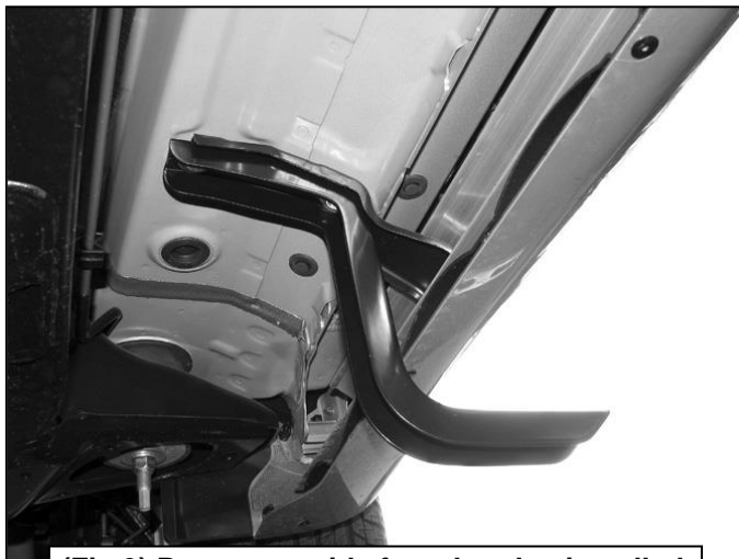
(Fig 3) Passenger side front bracket installed
