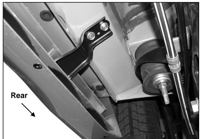
(Fig 4) Passenger side rear bracket location pictured
