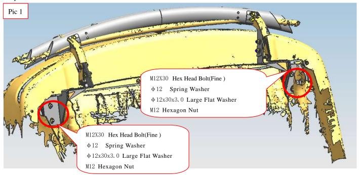
Step 3: Refer to Pic 2 and install the rear bumper on the brackets and adjust the rear bumper to the proper position.
