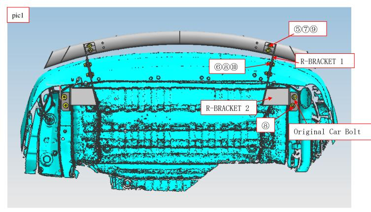
step3: Install the grille guard on the bracket and then adjust the installation position of the bracket according to the position of the grille guard.
