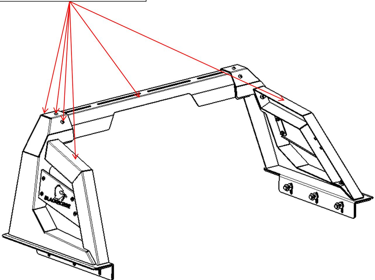
**Step2:** Place the roll bar on the truck in an appropriate location.
