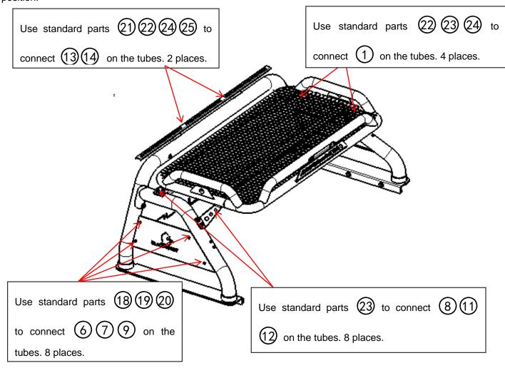
Step3: Put roll bar on the truck in an appropriate place. And use pen to mark the holes. 3 places in each part, 6 places total. Remove the roll bar then drill the size of  $\Phi$ 12 holes. Put the roll bar back and use standard  $\Theta$
