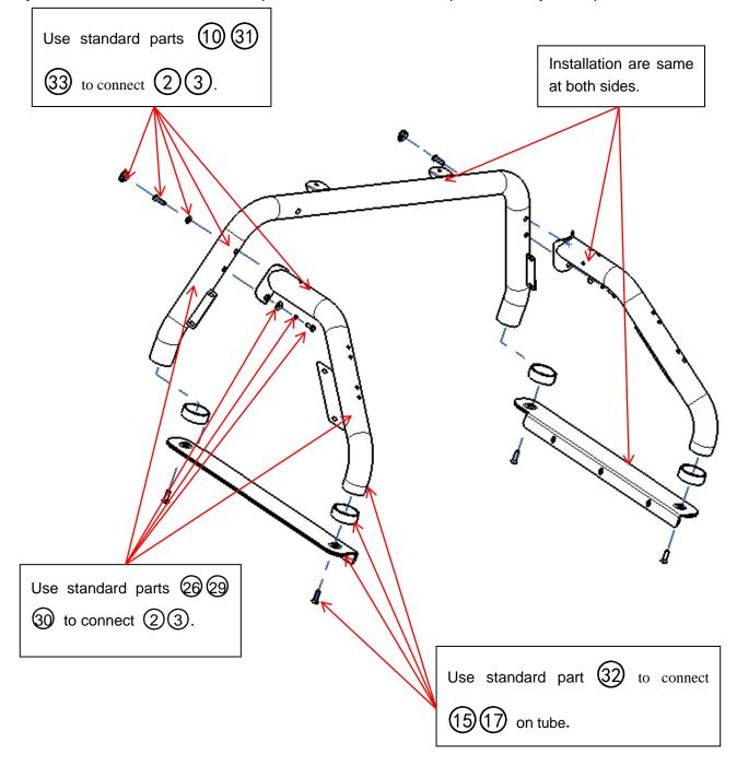
**Step2:** Assemble Luggage frame and tubes with standard parts. Lock all the standard parts after adjust the position.
