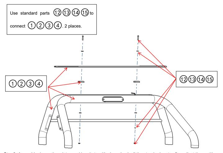
**Step2:** Assemble decoration plates and brackets with pipes. Lock all the standard parts after adjust the position.
