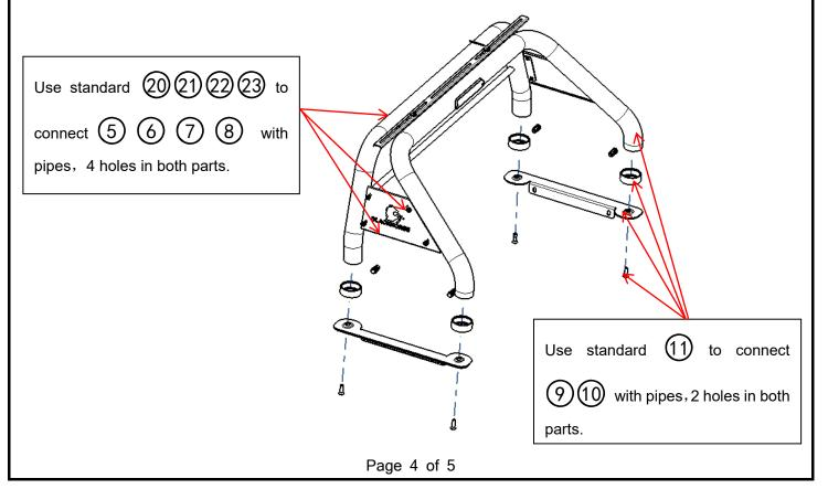
Step3: Put roll bar on the truck in an appropriate place. And use pen to mark the holes. 2 places in both parts, 4 places total. Remove the roll bar then drill the size of  $\Phi$  14 holes. Put the roll bar back and use standard (16)
