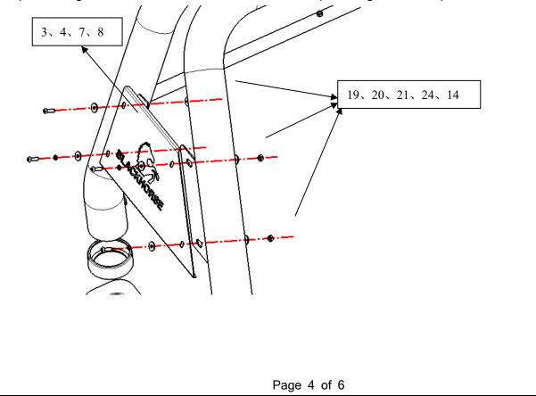
S/S UNIVERSAL ROLL BAR FOR 1/2 TON TRUCKS (GM SILVERADO 2015-FORD F150 2015) FLAT BASE WITH LED BRAKE LIGHT Step 4: Using wrench 13, install support plate 10 and gum cover 9 with part 26.
