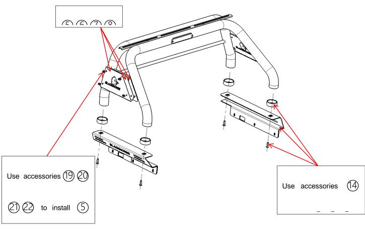
**Step3:** Place the roll bar on the truck in an appropriate location. And mark the hole with pen. 2 places in each part, total are 4 places. Remove the product.
