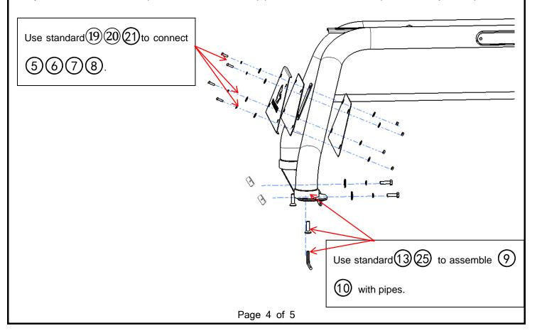
**Step3:** Fix the roll bar on the trunk with parts 12/14/16/17 (need to drill the trunk if there's no installation holes). Test and make sure that the roll bar is steadily fixed, and then tighten all the hardware.
