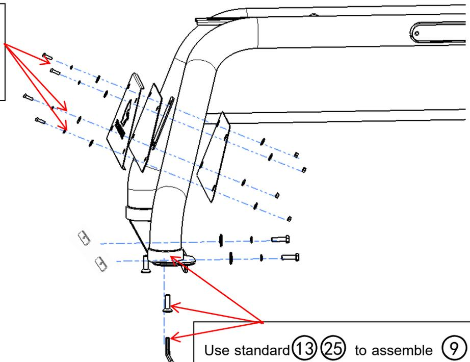
Use standard ⑬ ㉕ to assemble ⑨ ⑩ with pipes.
