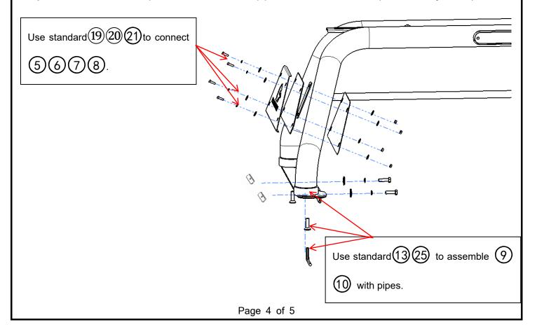
**Step3:** Fix the roll bar on the trunk with parts 12/14/16/17 (need to drill the trunk if there's no installation holes). Test and make sure that the roll bar is steadily fixed, and then tighten all the hardware.
