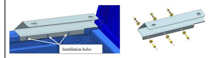
Step 6: Install the roll bar, mounting base and roll bar gum covers with standard part (9)
