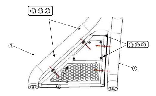
Step 4: After the preceding components are preinstalled, connect the side tube and middle tube with standard part ②.(To adjust tubes to appropriate position, lock tighten all accessories except standard part ②) PS: These adjustable holes can control the width of roll bar.
