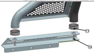
Step 7: Install the front and rear end cover with standard part (1), lock tighten all standard parts.
