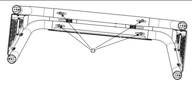
Step 5: Put mounting base(L/R) on both sides of the truck rail, to adjust the mounting base on suitable position, then mark down the installation holes for drilling(Ps: To make sure the drilling holes can go through with M10 standard parts). Install the mounting base on truck rail with standard parts 2000, as the following picture shown.
