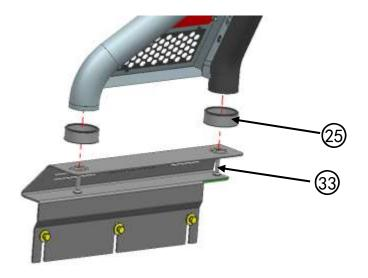
**Step 7:** Install the front and rear end cover with standard part 3.
