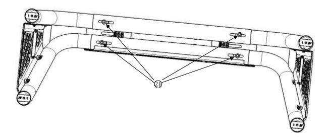
**Step 5:** Slip each 3 pieces plate nut  $\mathfrak{D}$  into both sides of utility side trail as the following picture shown, and put mounting base on the truck rail and adjust base to appropriate position, install them with standard parts  $\mathfrak{D}$   $\mathfrak{D}$  .
