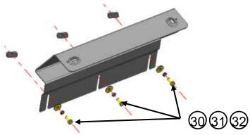
**Step 6:** Put the gum covers on each legs of roll bar, then install roll bar on mounting base with standard part 3. To adjust roll bra to appropriate position and lock tighten all standard parts.
