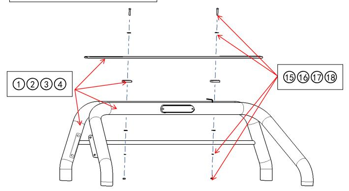
Step2: Assemble decoration plates and brackets with pipes. Lock all the standard parts after adjust the position.
