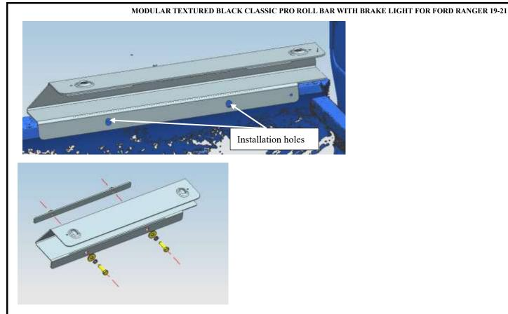
Step 6: Install the roll bar, mounting base and roll bar gum covers with standard part (3)
