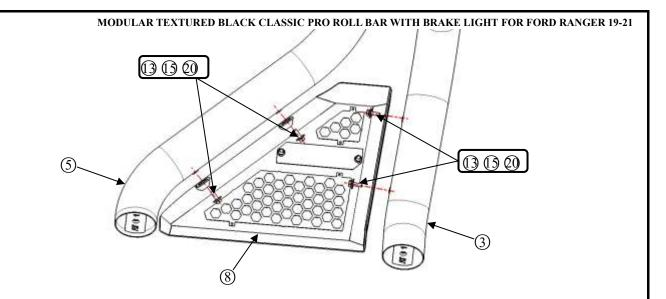
**Step 4:** After the preceding components are preinstalled, connect the side tube and middle tube with standard part  $\mathfrak{O}$ .(To adjust tubes to appropriate position, lock tighten all accessories except standard part  $\mathfrak{O}$ ) PS: These adjustable holes can control the width of roll bar.
