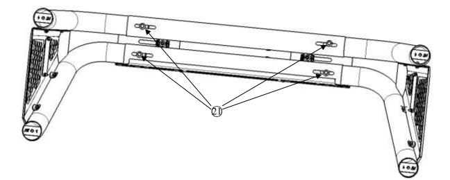
**Step 5:** Put mounting base(L/R) on both sides of the truck rail, to adjust the mounting base on suitable position, then mark down the installation holes for drilling(Ps: To make sure the drilling holes can go through with M10 standard parts). Install the mounting base on truck rail with Long plat nuts 29 and standard parts 32 33 34, as the following picture shown.
