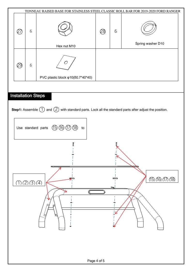
TONNEAU RAISED BASE FOR STAINLESS STEEL CLASSIC ROLL BAR FOR 2019-2020 FORD RANGER Step2: Assemble decoration plates and brackets with pipes. Lock all the standard parts after adjust the position.
