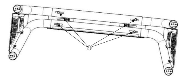
Step 5: Put 3 pcs 29 T bolt M10 and 30 10mm Plastic Retainer into the truck rail chute, and then put mounting base on suitable position. Install the mounting base on truck rail with standard parts 30 33, as the following picture shown.
