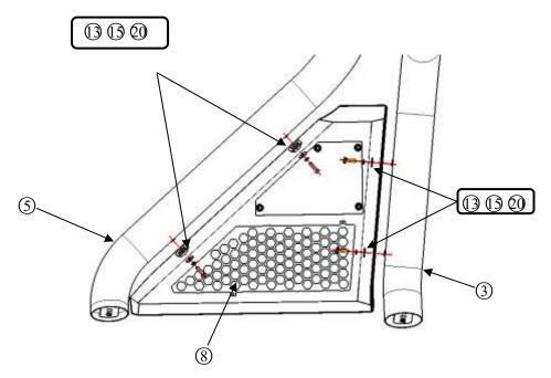
Step 4: After the preceding components are preinstalled, connect the side tube and middle tube with standard part ②. (To adjust tubes to appropriate position, lock tighten all accessories except standard part ②) PS: These adjustable holes can control the width of roll bar.
