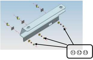
Step 6: Install the roll bar, mounting base and roll bar gum covers with standard part 3.
