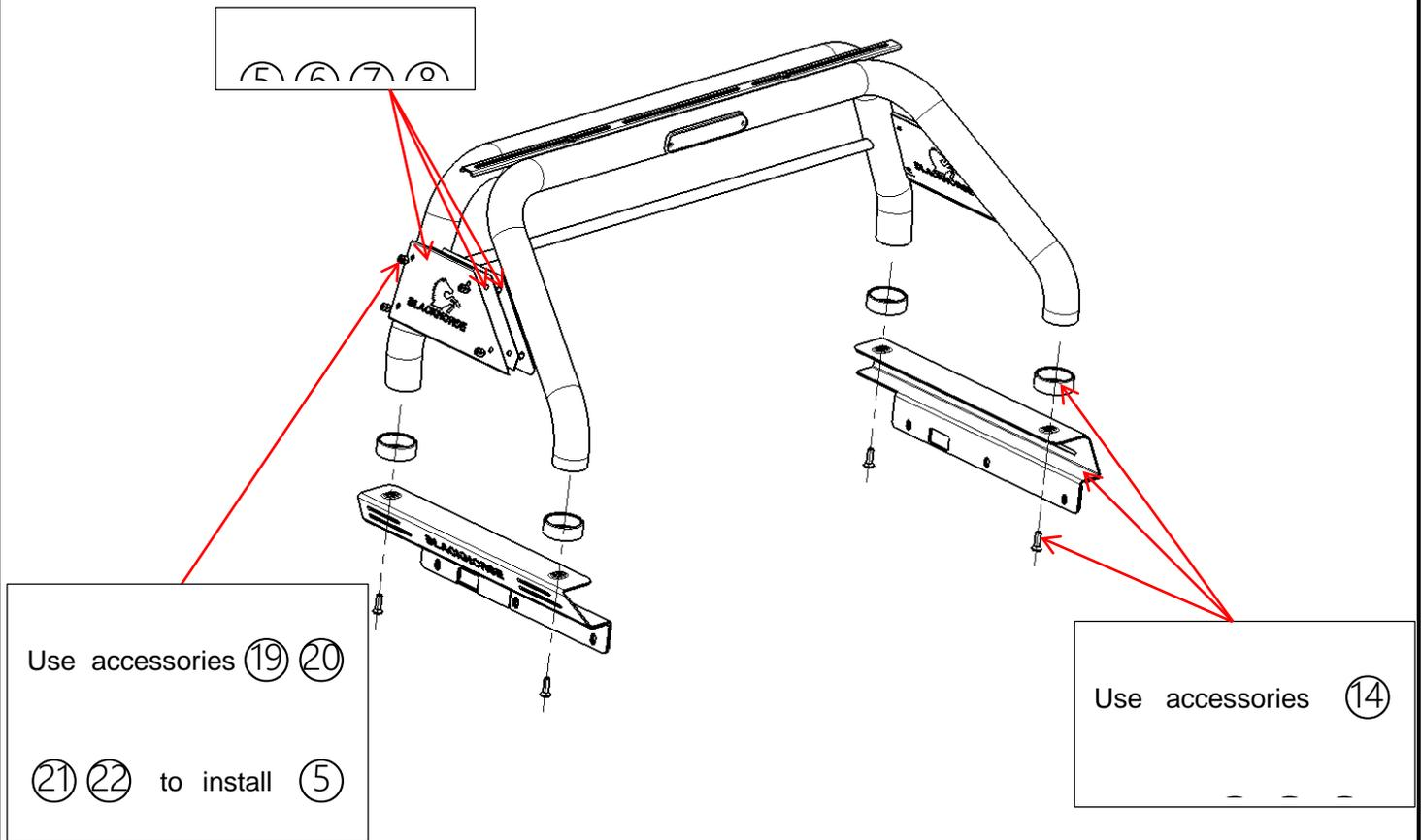
**Step3:** Place the roll bar on the truck in an appropriate location. And mark the hole with pen. 2 places in each part, total are 4 places. Remove the product.
