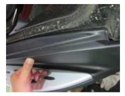
The top of the step cover should snap into the old rocker panel retaining clips , and also underneath the rocker panel there is a groove that will align the step cover ,so using your hands, align the underside of the step cover with the grooves and push it until you feel it snap into place.
