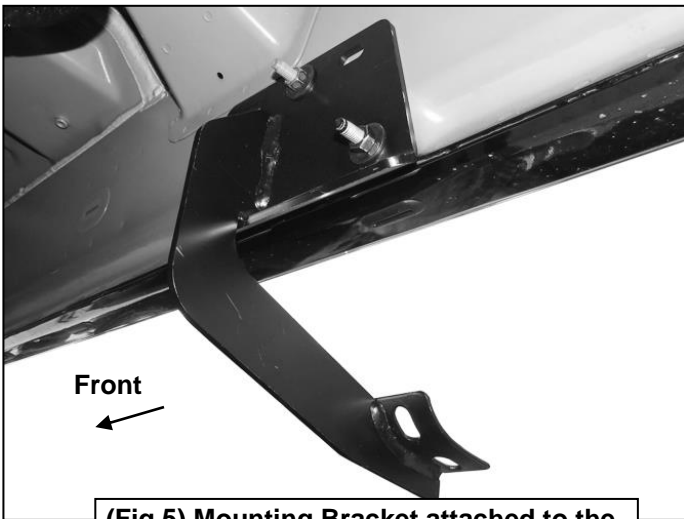
(Fig 5) Mounting Bracket attached to the passenger side center mounting location
